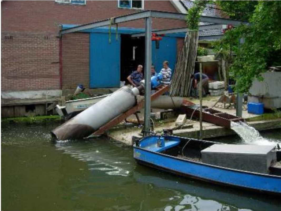
Figure 3.1 Test set up with screw pump
