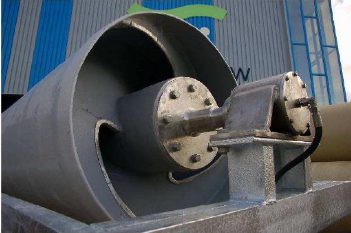
Figure 2.2 Screw pump of FishFlow Innovations
